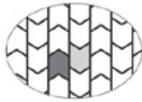
Broken Joint-2 Way
